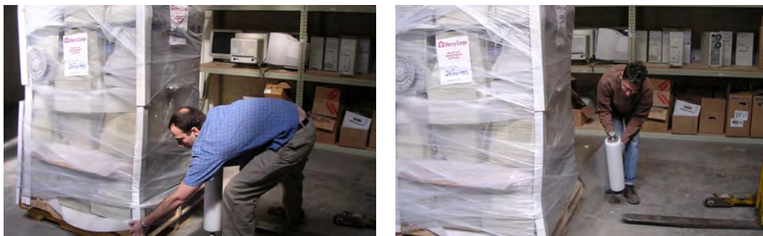
Fig 3.1.2: Packing heavy products using handling equipment
